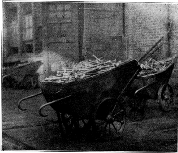
WAGONS FOR TRANSPORTING BOLTS IN BULK AT COLLINWOOD SHOPS., L. S. & M. S. RY.
